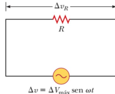
$$\Delta v = \Delta V_{\max} \sin \omega t$$
